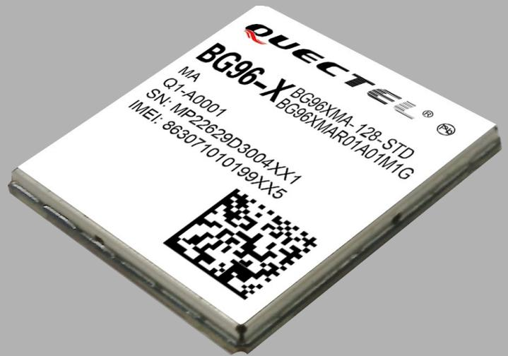
BG96 is a series of LTE Cat M1 and Cat NB1 module offering a maximum data rate of 375kbps downlink and uplink. It features ultra low power consumption, and provides pin-to-pin compatibility with Quectel LTE module EG95, NB-IoT module BC95, UMTS/HSPA module UG95/UG96 and GSM/GPRS module M95.
