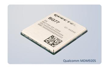
BG77 is an ultra-compact multi-mode LTE Cat M1/Cat NB2 module with integrated GNSS functionality. It is fully compliant with 3GPP Rel. 14 specification and offers a maximum data rate of 375Kbps downlink and 1.2Mbps uplink. It features ultra-low power consumption by leveraging the integrated RAM/flash as well as the ARM Cortex A7 processor supporting ThreadX, achieving up to 70% reduction in PSM leakage and 85% reduction in eDRX current consumption compared to its predecessor.
