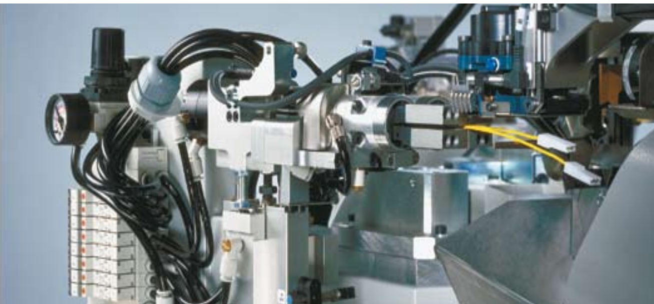
Double gripper module for horizontal and vertical connections
